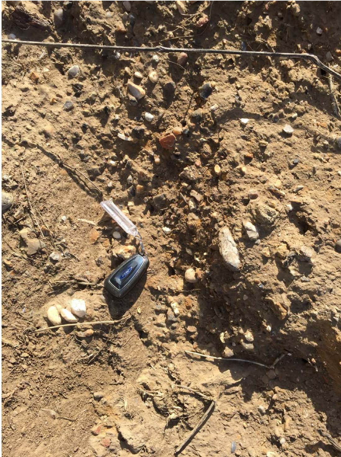
Figure 20. Silty gravelly SAND of the Glacigenic deposits with car keys (5cm length) for scale.
