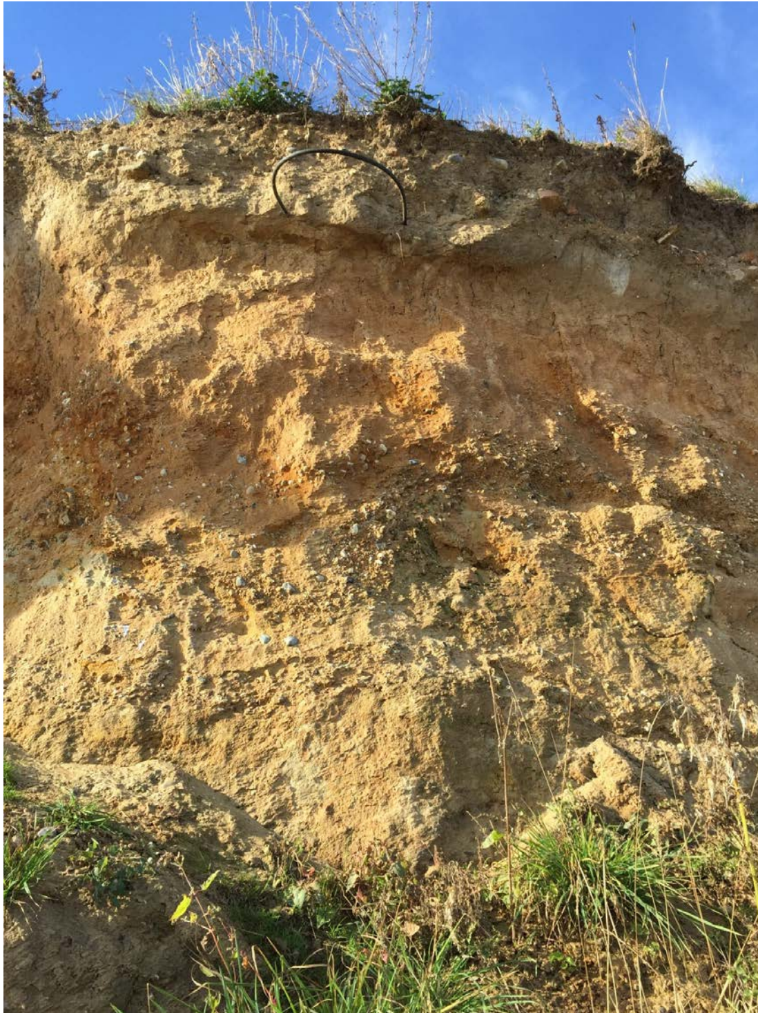
Figure 19. Cliff section at the northern end of the beach 20m beyond the low angle ramp. The Glacigenic deposits are silty gravelly SAND. The ground above the cable at the top of the cliff is head deposit or topsoil/made ground
