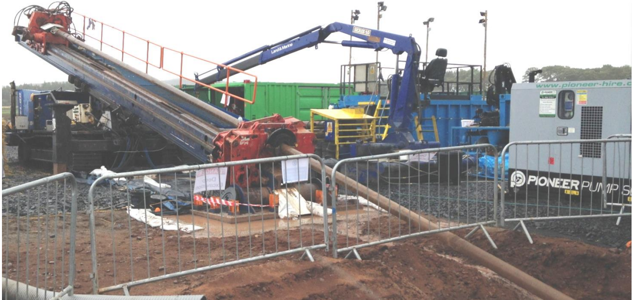
Figure 24. Example HDD rig of the maxi size likely to be used for the long HDD's.
