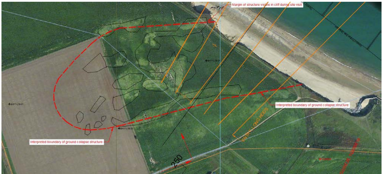
Figure 5. Estimated margin of ground subsidence structure indicated by red dashed line. Black lines indicate topographical variations interpreted from 1946 aerial photograph. The orange lines indicate potential routes for HVAC cable HDD's.
