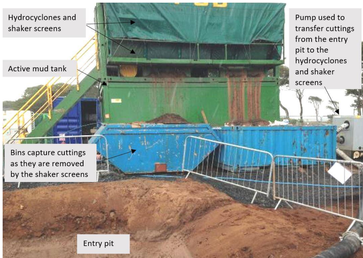
Figure 27. A drilling fluid recycling unit with components indicated.
