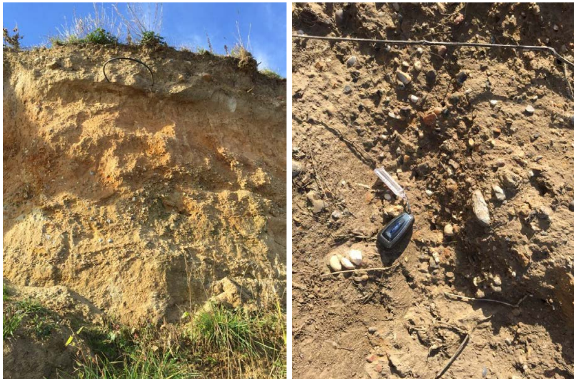
Figure 2. Glacigenic deposits exposed in the cliffs just north of the potential drilling alignment. These figures are also provided at larger scale in Appendix C.
